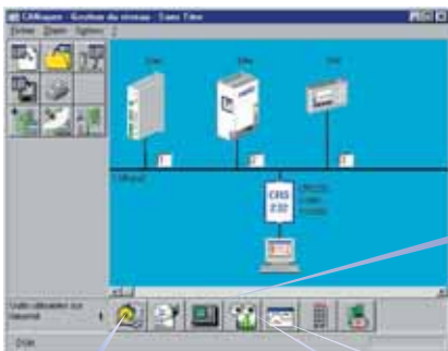
CANopen or PROFIBUS network management Simple click access to all subscribers on network.
