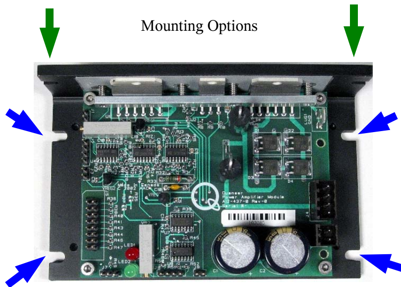
Figure 14. Mounting hole locations A (green) or B (blue).
