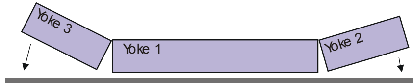
Figure 9: Principle of controlled rotational mounting of the magnet yokes
