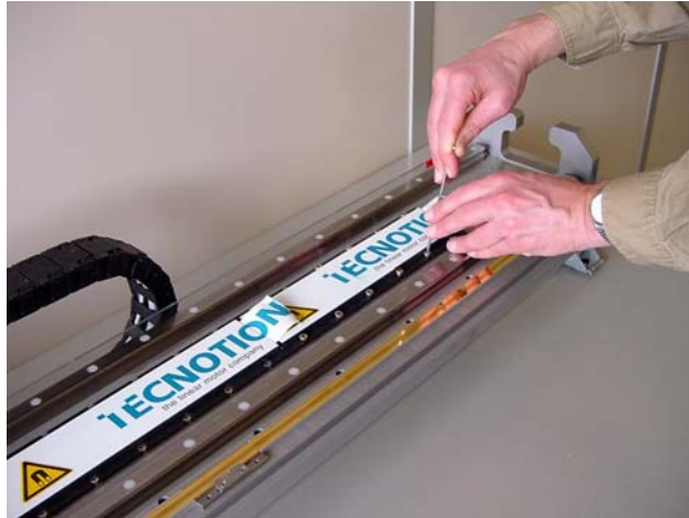
Figure 7: Installing a linear motor system
