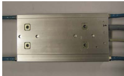
Figure 24: TL-water-cooling with four connection points
