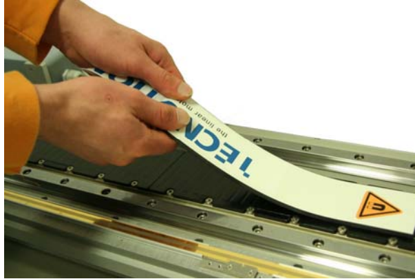
Figure 16: Uncovering the magnet track
