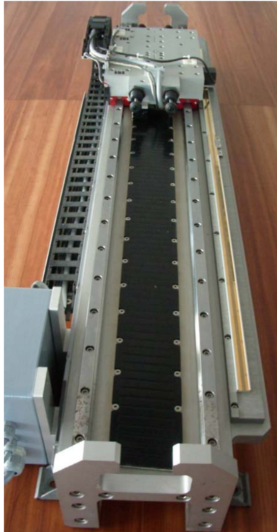
Figure 1: A complete iron core linear motor system
