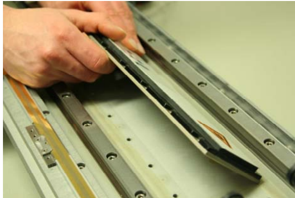
Figure 12: Orientating the magnet plates
