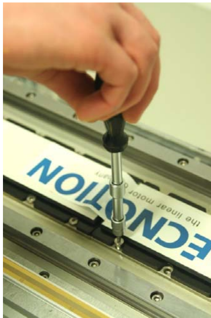
Figure 13: Mounting the Magnet plates
