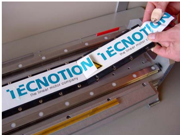
Figure 15: Placing another magnet plate
