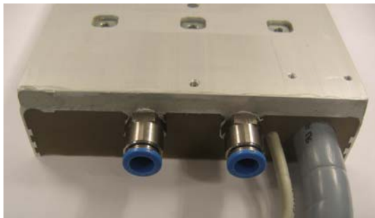
Figure 23: TBW-water-cooling with two fittings
