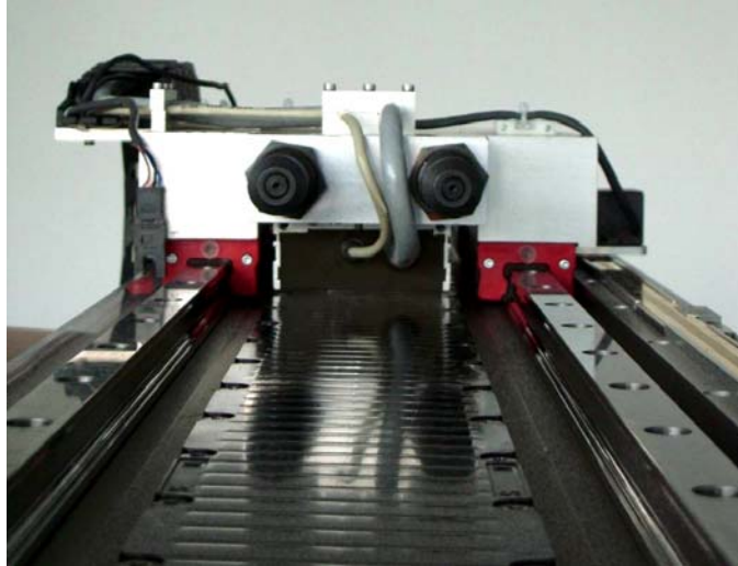
Figure 23: Ironcore motor, sledge, bearings and ruler, detail
